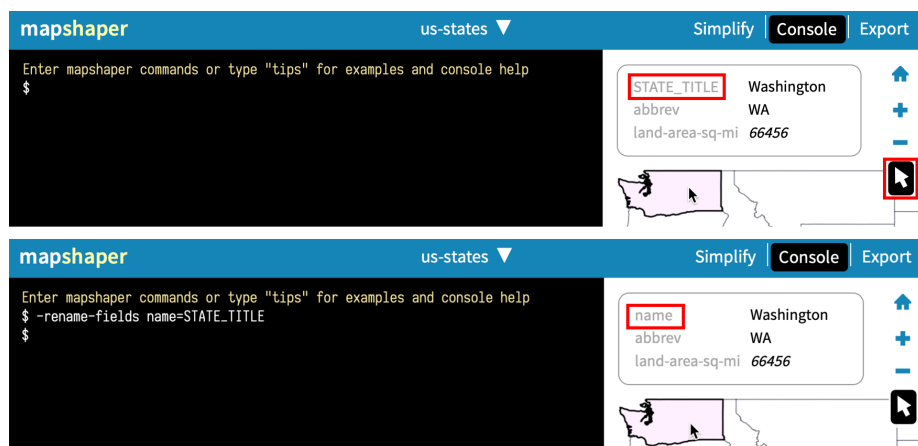
Figure 13.10: Select the Inspect Features arrow to view field names, and rename them using the -rename-fields command in the console.
