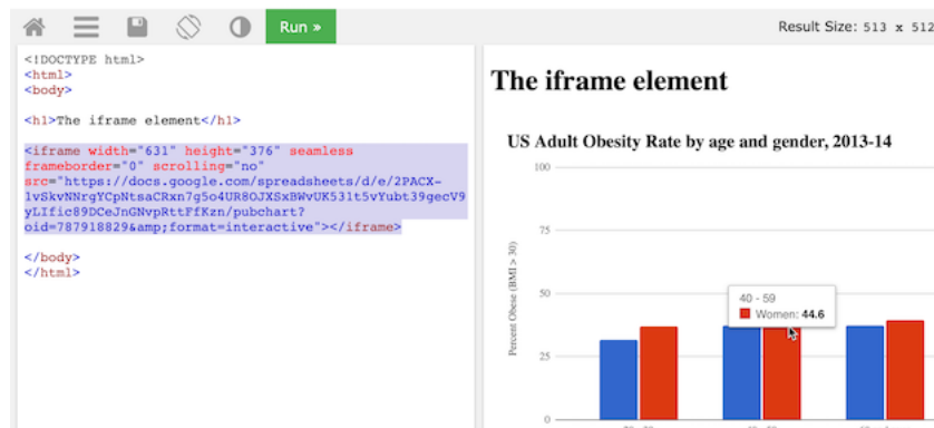
Figure 9.6: Paste your Google Sheets embed code to place of the current iframe tag in the TryIt page and click Run .
